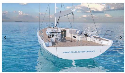
The **deck plan** and **sail plan** are designed differently in the two versions: the "Performance" version features an "easy sailing" deck plan with 4 winches at the stern, a standard self-tacking jib and standard carbon bowsprit; the cockpit is not involved in any manoeuvres so that it can be safely used by guests. The "Race" version, however, features 6 winches, longitudinal rails for the jib, rlarger sail plan and a carbon bowsprit that is 90 cm longer than the standard version.
