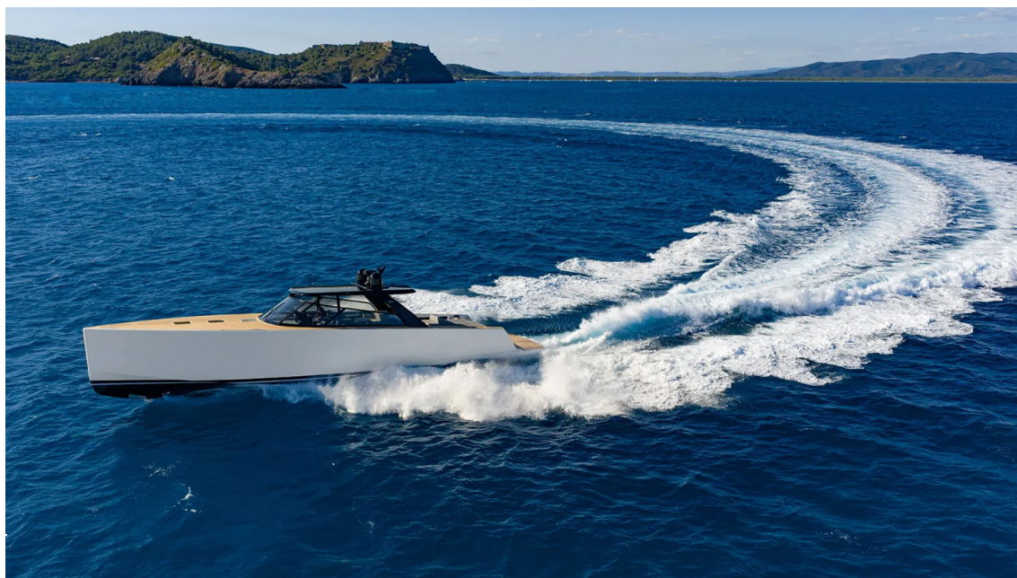
Triple Volvo Penta IPS drives push the VanDutch 75 to 40 knots with a cruising speed just a touch below that
